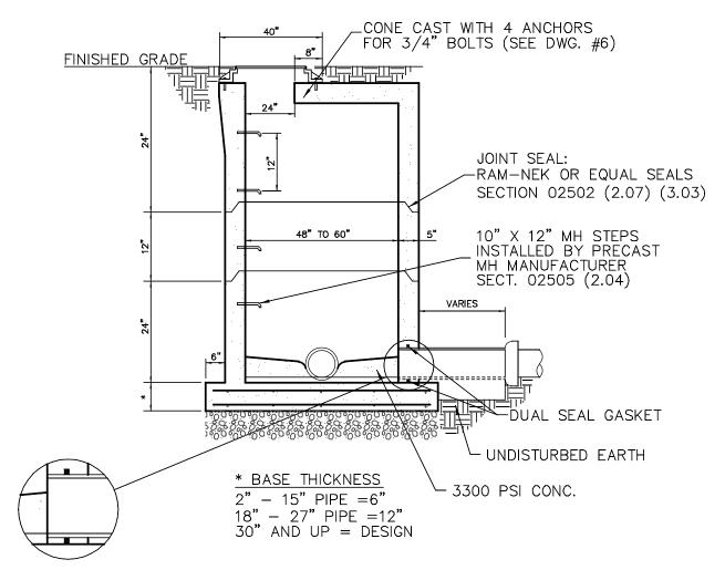
A-LOK GASKET WATERSTOP PER ASTM C923 CAST INTEGRALLY IN MANHOLE WALL JOINT ALLOWS 10" OMNIDIRECTIONAL DEFLECTION SECTION 02505 (2.06)
