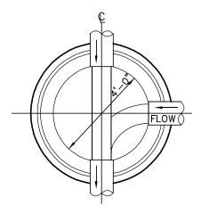
NOTE: ALL BENCHES SHALL SLOPE A MINIMUM OF 2" PER FOOT TOWARD FLOW CHANNEL
